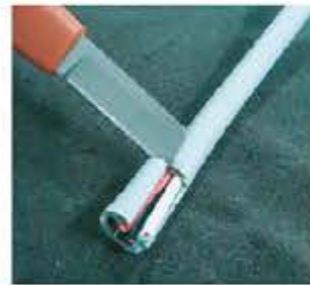
For stripping cable
